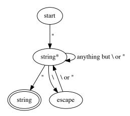
Figure 1: A finite-state machine for lexing a Scheme string.
